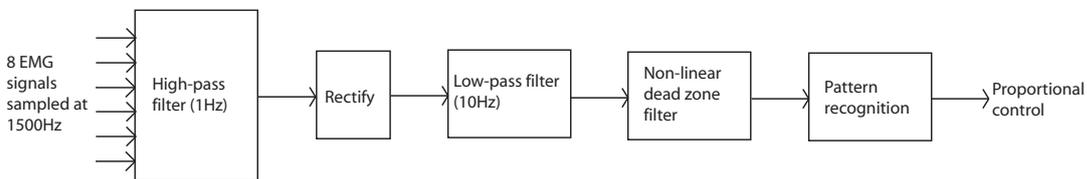
**Figure 12:** Proportional control system based on EMG signals
