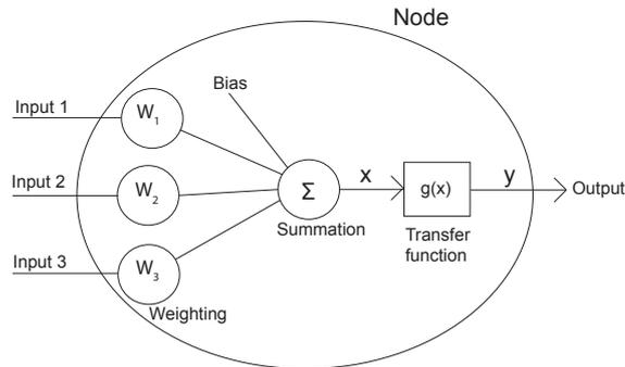
**Figure 10:** Example of a single node in a MLP network
