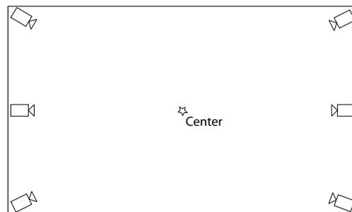
**Figure 3:** VICON camera placement
