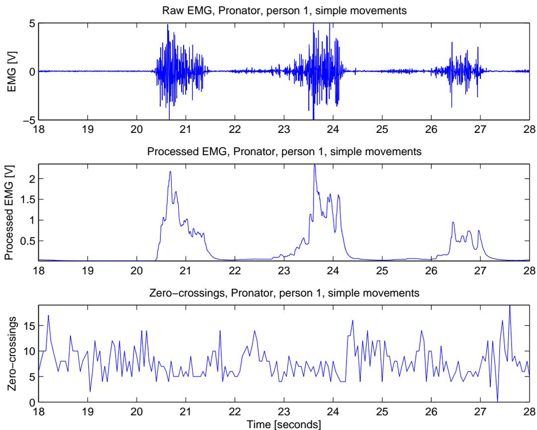
Figure 13: EMG processing example, channel 1 (Pronator), person 1
