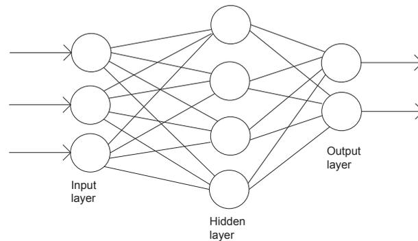
**Figure 9:** Example of MLP network with 3 inputs, 2 outputs and 4 nodes in the hidden layer
